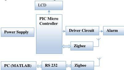
Figure 11: Overview of hardware block diagram
