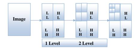
Figure 2: Discrete wavelet transforms (2D-DWT) operation
