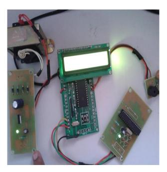
Figure 13: ZigBee Receiver
